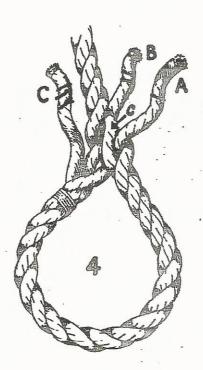
For Step 4, turn the partially completed eye over and tuck C under c. By checking you will find that there is only one strand in the standing part under which no tuck has been made. After C is so tucked, pull it snug to the seizing. If you are correct you will find each strand of the standing part between 2 strands of the working end.
