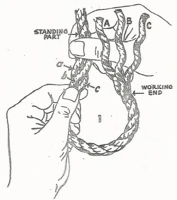
Looking at Step 2, B is now tucked under b, and is pulled snug to the seizing. In Step 3, A is tucked under a and pulled snug to the seizing.
